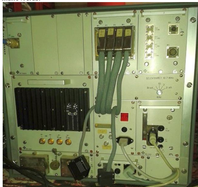
Fig 5 Mottagarrack EV1260/H å Stureby Radio (vikt 47 kg)
