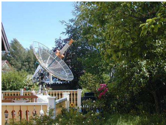
SM5LE 2.2 m parabol (1296 MHz)
